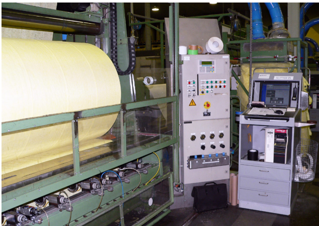
One of 18 workstations equipped with scanner, screen and label printer that sit next to a slitter machine in PGI's manufacturing department.
